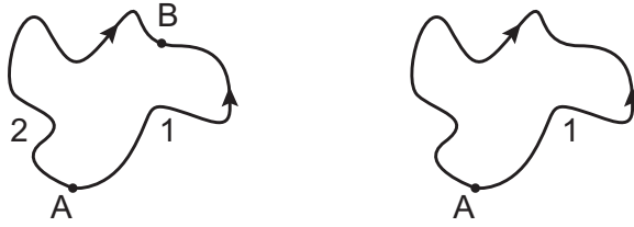
Figure 5.2 Illustration of Anderson localization in loops. (a) The probability to go from A to B via path 1 (amplitude P_1 ) or path 2 ( P_2 ) is \propto P_1^2 + P_2^2 , without interference terms because all contributing fields have a random phase. (b) Only paths returning to A always interfere constructively with their reversed counterparts, resulting in a return probability \propto (P_1 + P_1)^2 = 4P_1^2 .
