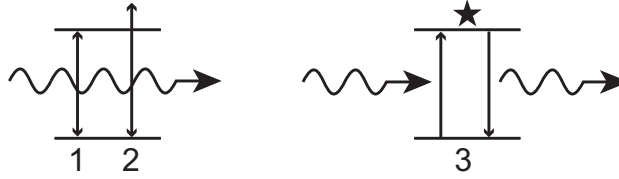
Figure 1.2 Comparison of (coherent) scattering and (incoherent) fluorescence in an energy diagram. Light may scatter off a two-level atom by resonance fluorescence (1). If there is more internal structure to the atom also Rayleigh scattering (2) is possible. Light may also be absorbed and re-emitted in fluorescence (3), in which the energy is stored in an atomic excitation (★) for some time.
