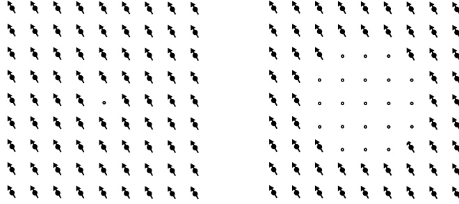
Figure 2.2 Two spherically symmetric subsets of dipoles on a cubic lattice: Left the subset \{\mathbf{R} \neq 0\} , right \{\mathbf{R}_{\text{out}}\} , corresponding to Eqs. 2.39 and 2.37, respectively. Both subsets are captured by \{\mathbf{R}'\} .
