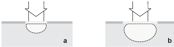
figure 3.2 Form of the inversion profile. a) at low pumping energy, b) at higher pumping energy. The dimensions of the gain volume become larger when the pumping energy is increased. Probe light will be amplified in a larger volume and the effective surface from which the light emerges is expanding. From outside the medium this is observable as an increase of the source dimensions, which is indicated by the light-coloured part of the surface.
