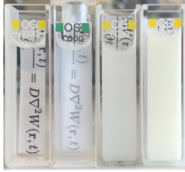
Figure 1.2: Light scattering in a suspension of milk with different concentrations inside four cuvettes. From left to right, the content of the cuvettes are water, milk suspension diluted 500 times, milk suspension diluted 50 times, and undiluted milk suspension. Behind each cuvette is the diffusion equation printed on a white paper.
