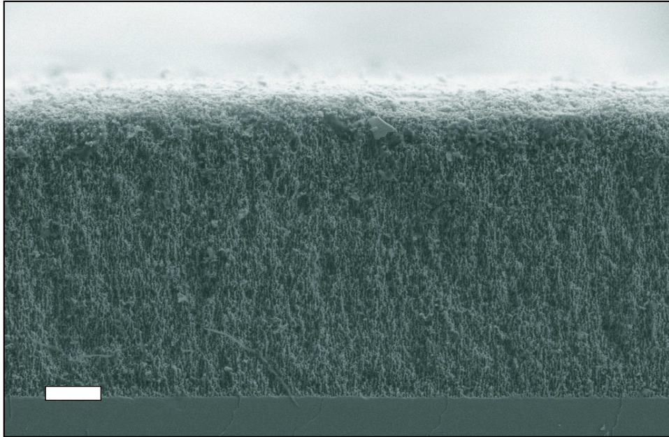
Figure 4.2: SEM picture taken from the side of the porous GaP layer of Sample 2. The white scale bar is 4\text{ }\mu\text{m} .
